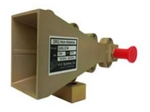
The SAS-574 Double Ridge Guide Horn Antenna is a broadband antenna that offers excellent performance over the frequency range of 18 GHz to 40 GHz. The original design was to have a 30-degree beamwidth, which is ideal for EMI measurements and compliance testing.
