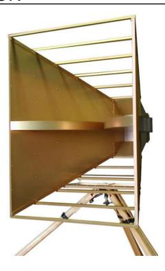
The SAS-570 Double Ridge Guide Horn Antenna is lightweight, compact and has been manufactured for maximum gain, low VSWR and broadband response. The SAS-570 is a linearly polarized broadband antenna that covers the frequency range of 170 MHz – 3 GHz and is typically used to generate high RF fields with relatively low input power. With the high gain characteristics of the SAS-570, this antenna can also be used for receiving low signals.
