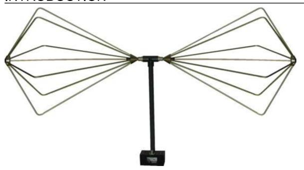
The SAS-544 Biconical Antenna is designed with a coaxial wound balun for increased power capability and intended for both transmitting and receiving high electromagnetic RF fields. This Biconical antenna may be used for radiating immunity measurements. Whether testing in a shielded enclosure, or outdoors, the rugged construction of the A.H. Systems Biconical antenna will ensure long life, and reliable performance.
