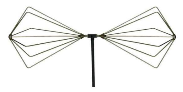
The A.H. Systems SAS-540 Biconical antenna operates efficiently over the frequency range of 20 MHz to 330 MHz. Compact in size, this Biconical Antenna is an ideal for use in a shielded room or anechoic chamber. The antenna balun is designed using as unbalanced to balanced transformer for improved linearity response and is the standard workhorse of any EMC compliance test house.
