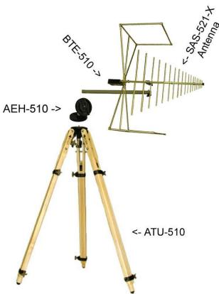
Mount the antenna such that the elements are parallel to the ground for horizontal polarization testing, or perpendicular to the ground for vertical testing. The horizontal beamwidth of the Bilogical is approximately 45 degrees and it should be pointed or aimed in the direction that the received signal is coming from.
