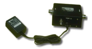
The PAM-0118P broadband preamplifier is an excellent choice for improving system dynamic range. The performance of this preamplifier will increase your system sensitivity by at least 35 dB and is ideal for low-amplitude test measurements. When measuring in the EMC lab or out in the field for general RFI testing, this preamplifier has a rugged compact design.
