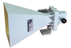
$\begin{array}{rll} \mbox{Frequency Range:} & 4 \mbox{ GHz} - 8 \mbox{ GHz} \\ \mbox{Antenna Factor:} & 30 \mbox{ dB typical} \\ \mbox{Gain:} & 15.5 \mbox{ dB typical} \\ \mbox{Maximum CW Power:} & 200 \mbox{ Watts} \\ \mbox{Max Radiated Field:} & 500 \mbox{ V/m} \\ \mbox{Impedance:} & 50 \mbox{ \Omega} \\ \mbox{VSWR:} & 1.2:1 \mbox{ (1.5:1 max)} \\ \mbox{Connector:} \mbox{ WR-159 to N-Type female adapter} \end{array}$
