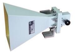
$\begin{array}{rll} \mbox{Frequency Range: } 2\mbox{ GHz}-4\mbox{ GHz}\\ \mbox{Antenna Factor: } 24\mbox{ dB/m typical}\\ \mbox{Gain: } 15.5\mbox{ dBi typical}\\ \mbox{Maximum CW Power: } 300\mbox{ Watts}\\ \mbox{Impedance: } 50\mbox{ } \Omega\\ \mbox{VSWR: } 1.2:1\mbox{ (1.5:1 max)}\\ \mbox{Connector: } WR-320\mbox{ to N-Type female adapter}\\ \end{array}$
