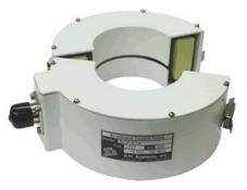
Frequency Range: 10 KHz - 300 MHz Transfer Impedance (dBΩ): -25 to 2 Max Cont. Current: 500 Amps (DC to 400 Hz) Peak pulse Current: 100 Amps Connector: N-Type, Female
