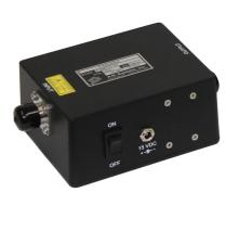
In the setup, avoid exposing the preamp to strong EMI or RF signals that could induce additional noise. Use enclosures when practical.
